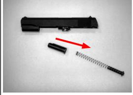
4.REMOVE THE BARREL BUSH AND **BARREL**
