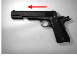
3.REMOVE THE RECOIL SPRING AND SPRING CAP
