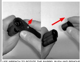
USE WRENCH TO ROTATE THE BARREL BUSH AND REMOVE ΙT
